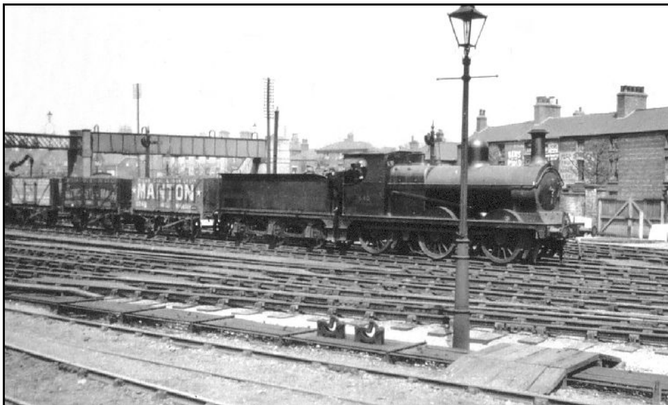
A class J10 0-6-0, still with its GC number painted on the cab side, heads east out of Lincoln Central on the through road with a string of private-owner mineral wagons. The first, belonging to Manton Colliery, looks like new. The date is 9th May 1924. Both the Parker class 9D and the Pollitt/Robinson class 9H were classified as class J10 by the LNER. The position of the lamppost makes for an unusual composition!
