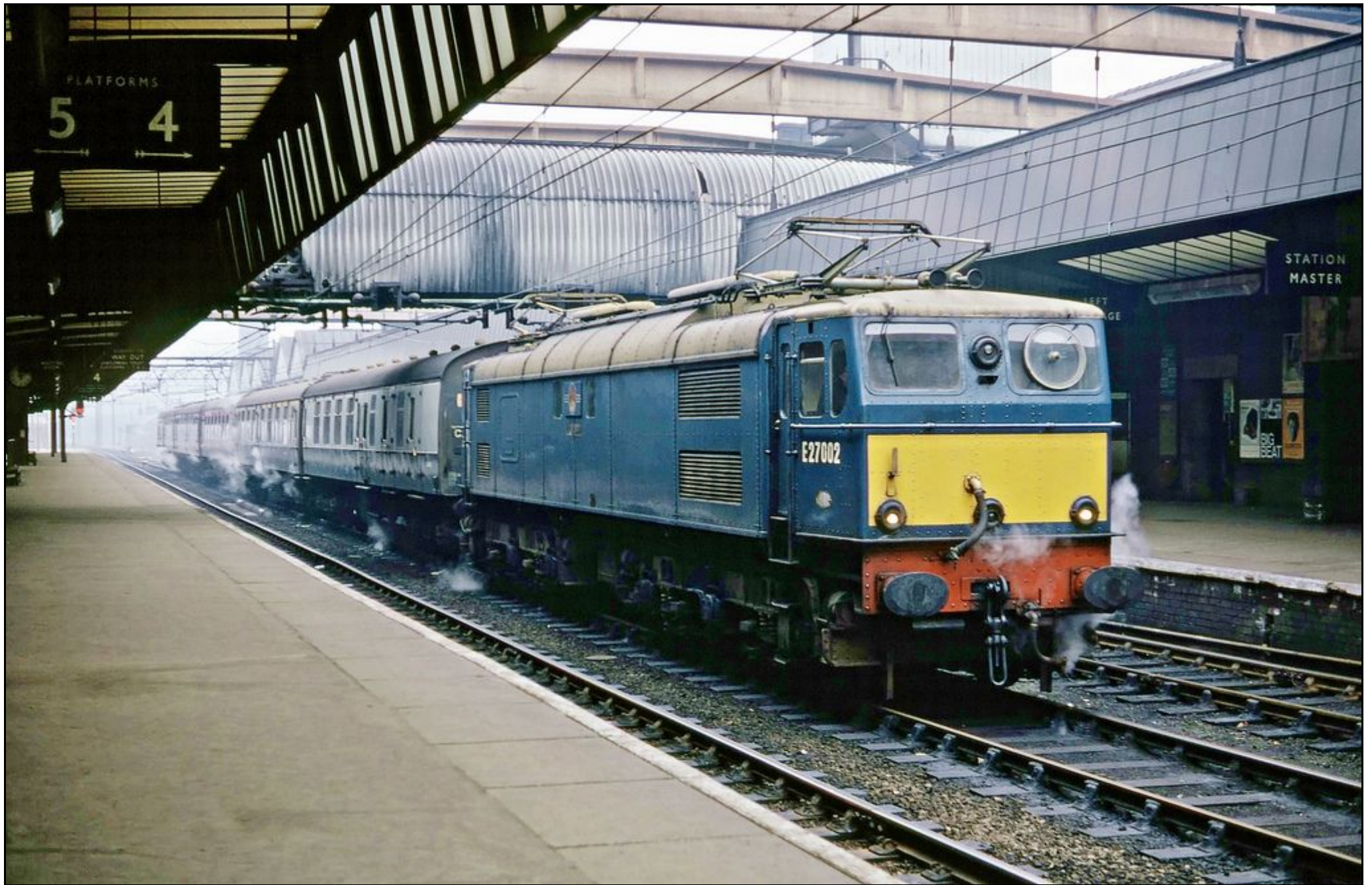
'Aurora' at Sheffield Victoria. Class EM2 Co-Co no. E27002 Aurora steam heats the stock for the 11.45am to Manchester in the centre road at Sheffield Victoria. The nameplates and builder's plates have already been removed from the locomotive. (Where are they now?). The addition of the circular windscreen wiper has created a strange monocoed effect. Was this unique to 27002? The date is 21 Feb 1968. photo: Bill Wright
