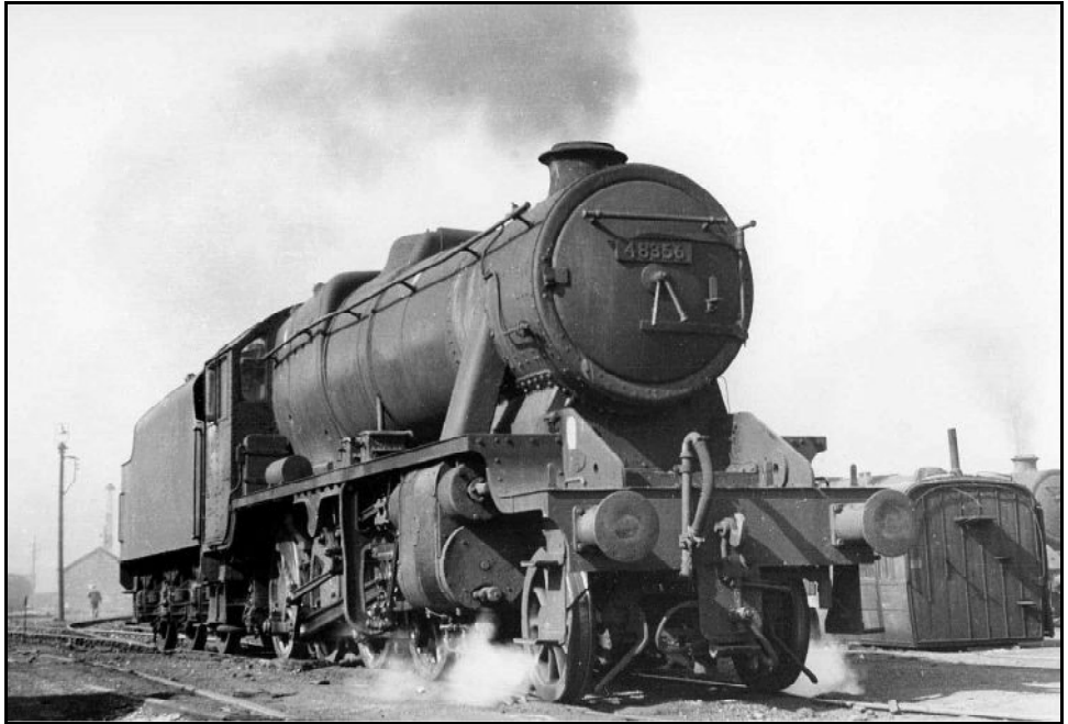
BR Stanier 8F 2-8-0 no. 48356 stands alongside the shunters' cabin at Annesley Yard in May 1965. The much respected O1s were replaced by the Stanier 8Fs in 1962.
