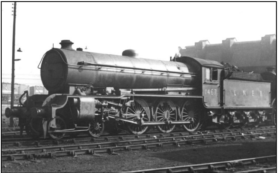
B16/3 4-6-0 no.1467 resting on shed at Darnall after being serviced and awaiting its return to the north-east on the Bournemouth-York in March 1948. This was a Thompson rebuild of Raven's NER design with three Walschaerts gears. photo: Rail Archive Stephenson
